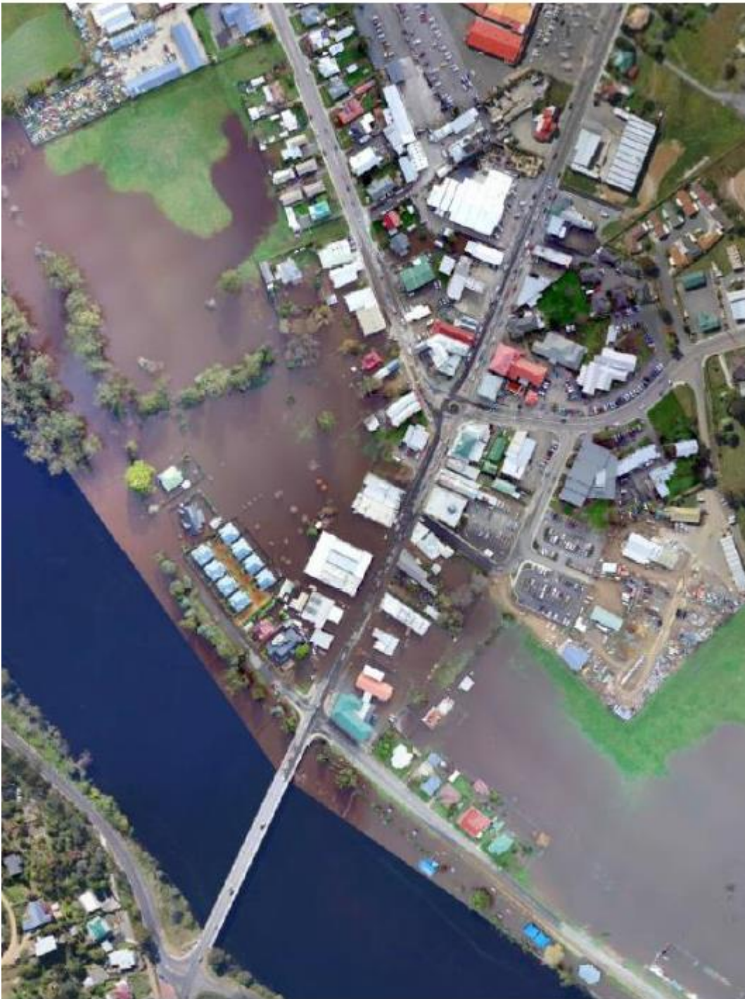
2016 flood event: source: Huon Valley Council, Gauge height at Huonville 4.1m est 5-10% AEP
